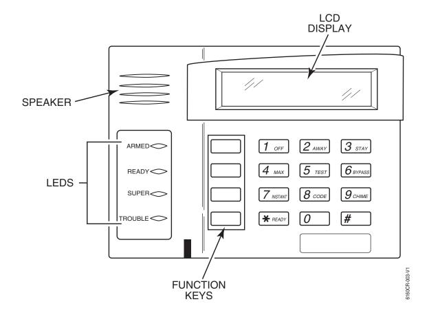
**IMPORTANT!** When using the keypad to enter codes and commands, sequential key depressions must be made within 3 seconds of one another. If 3 seconds elapses without a key depression, the entry is aborted and must be repeated from its beginning.
