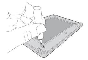
Install the screw into the LOCK position on the left. This locks the hinged door on the GC3e Control Panel.
