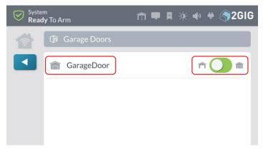
At the Garage Door screen press the toggle to open or close the Garage Door.
