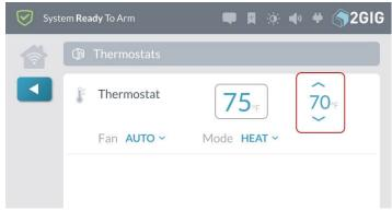
To change the temperature set points, press the top arrow to raise the temperature or press the bottom arrow to lower the temperature.
